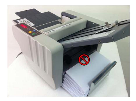
3.6 Press START/STOP button to run the machine. Machine will stop automatically if sheets run out. You can also press START/STOP button again to stop the machine at any time.
